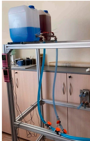
Figure 9. Laminar flow of coolant during the measurement of its flow time through the alternative short section of plastic pipe replacing the oil-cooler.
