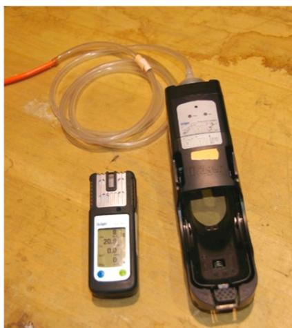
**Figure 2.** Photograph of Dräger X-am 5000 hand-held meter and air sample tubing.
