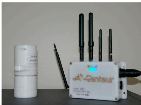
**Figure 1.** Photograph of the wireless sensor on the left and communication electronics on the right.
