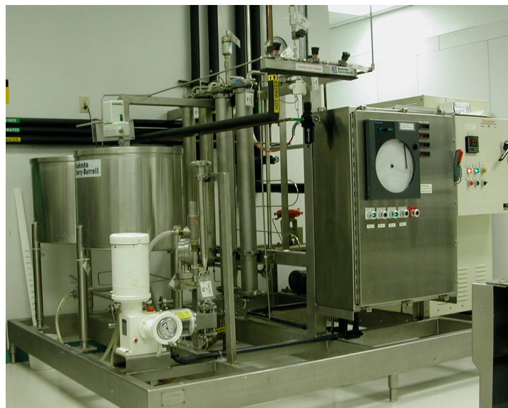
Figure 1. Frontier Scientific's flash sterilization system used for the processing of insect media. From left to right: diet tank, pump, processing tubes, coiled spiralthermers, and control station.
