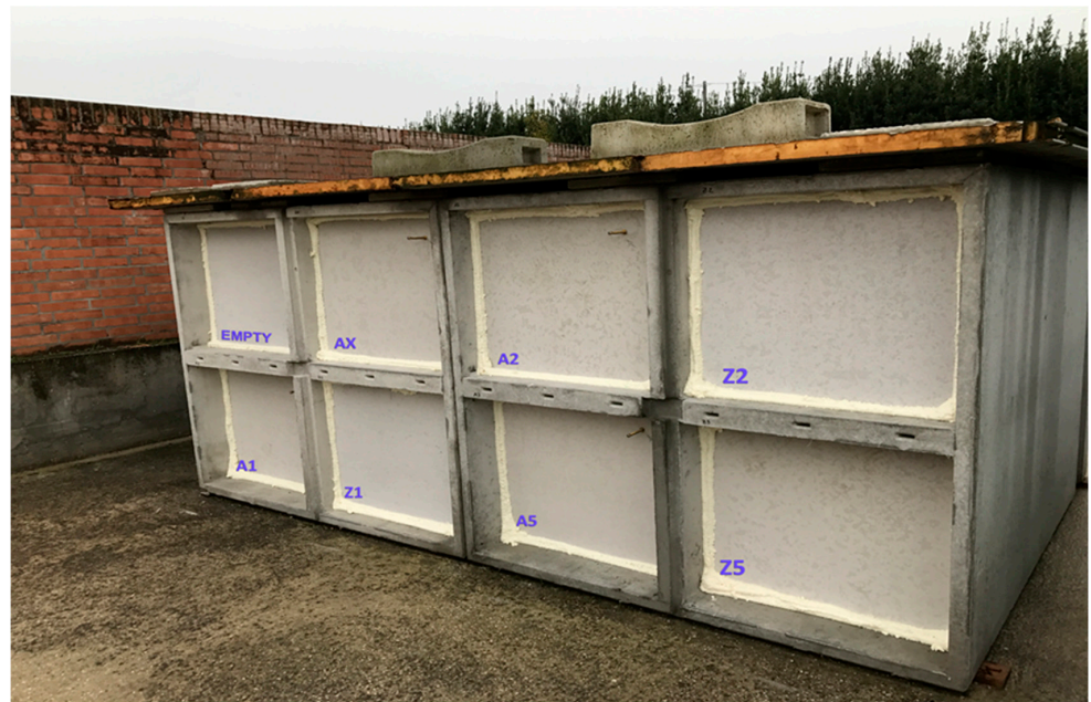
Figure 1. Structure of different burial niches (A = Aerated niche; Z = Watertight niche) (dimensions 230 × 80 × 80 cm).
