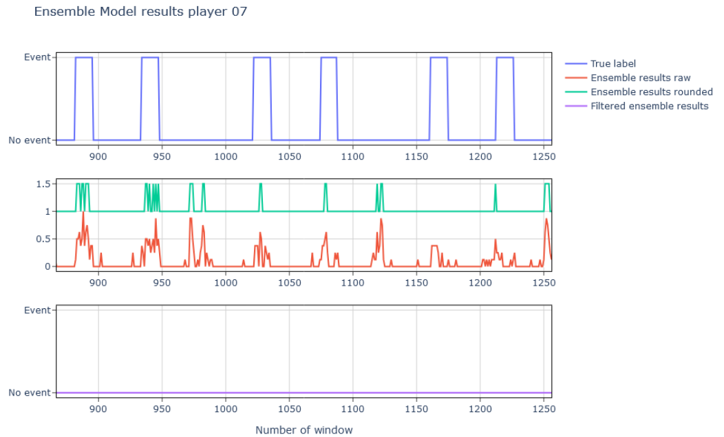
Figure 16. Representation of the true labels, the results of the ensemble model (the raw averaged results in red and the rounded averaged results in green), and the final predictions after filtering out those with insufficient duration.
