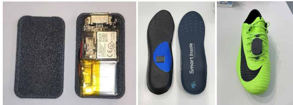
Figure 2. (left) IMU Sensor. (middle) IMU Sensor placed inside the insole. (right) IMU Sensor placed on the instep.
