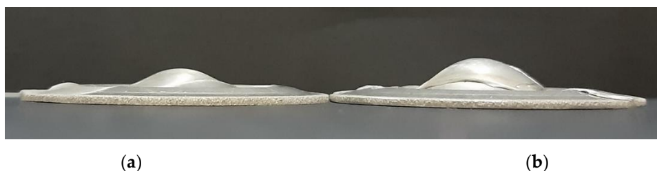
Figure 8. FSWed samples, tested at punch speed of 4500 mm/s, with different dome heights: (a) onset of necking (dome height of 4.0 mm), and (b) failure region (dome height of 4.5 mm).
