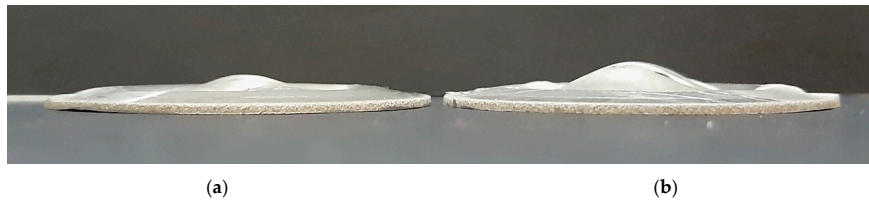
Figure 9. FSWed samples, tested at a punch speed of 0.1 mm/s, with different dome heights: (a) onset of necking (dome height of 3.3 mm) and (b) failure region (dome height of 3.8 mm).
