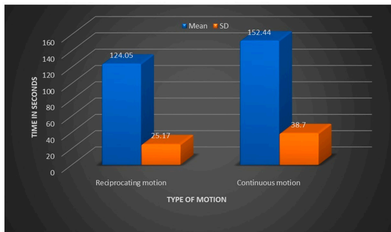
Figure 4. Comparison of mean time to fracture files with different motion files.
