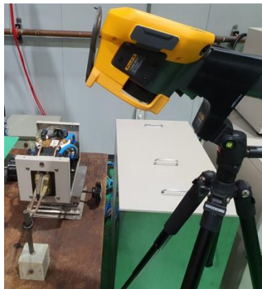
Figure 1. Measurement temperature setup for the AISI 1045 specimen during induction heating.
