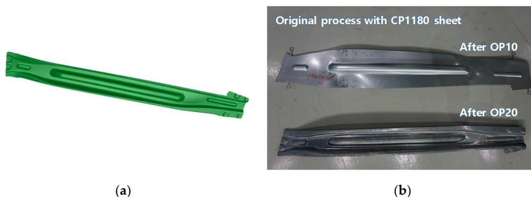
**Figure 11.** Target door impact beam: (a) Modeling of the target door impact beam; (b) Original process (OP10 and OP20) with CP1180 sheet.
