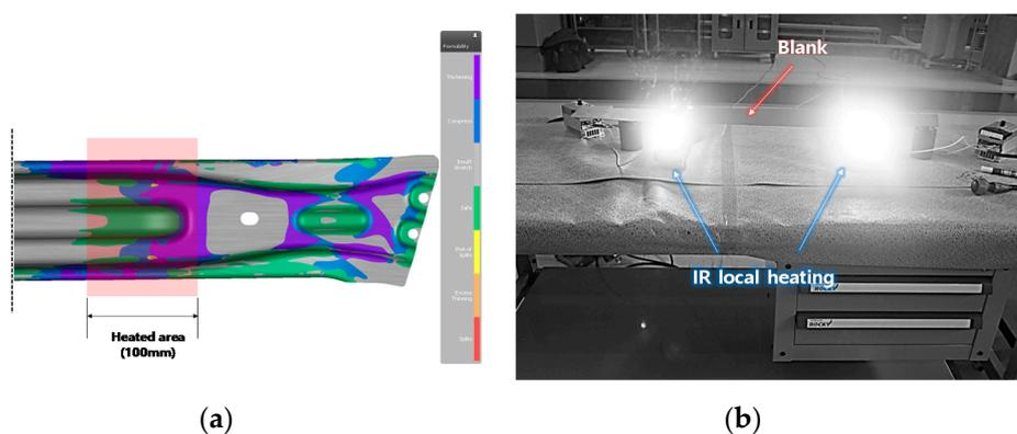
**Figure 12.** Heat treatment for the door impact beam application: (a) Heat treatment area on the left side of the door impact beam; (b) Heat treatment process.
