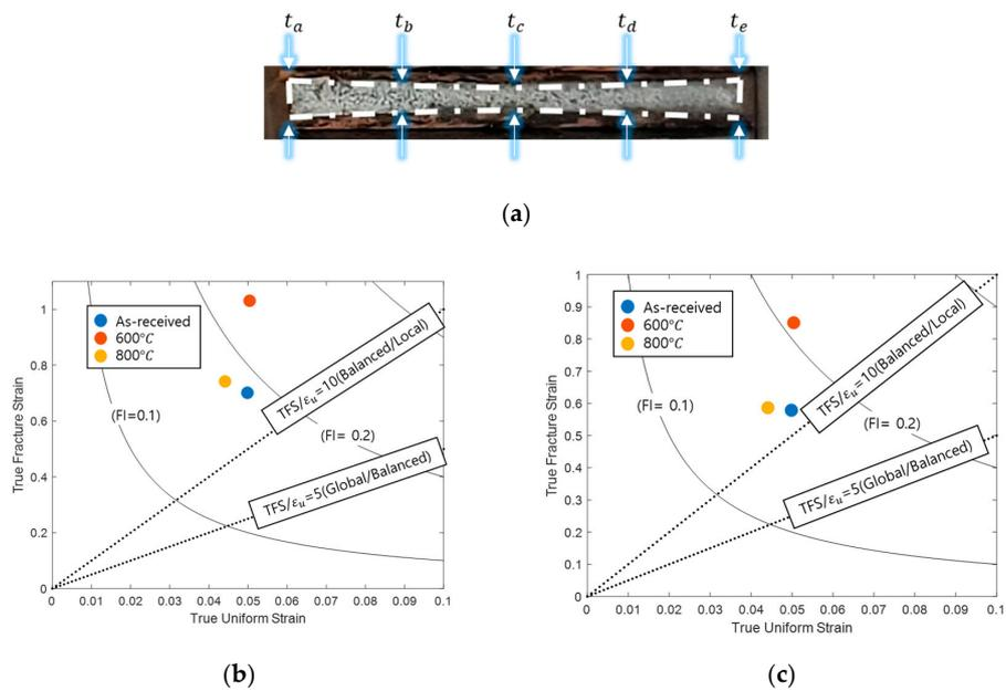
**Figure 10.** Local formability: (a) Cross section of a fracture specimen after the tensile test; (b)  $TFS_{area}$ ; (c)  $TFS_{thickness}$ .
