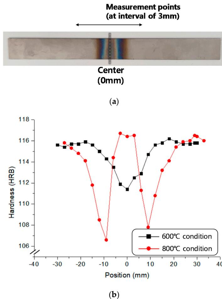
Figure 8. Hardness distribution of the 600 and 800 °C-heat-treated specimens: (a) Hardness measurement setting; (b) Hardness distribution.
