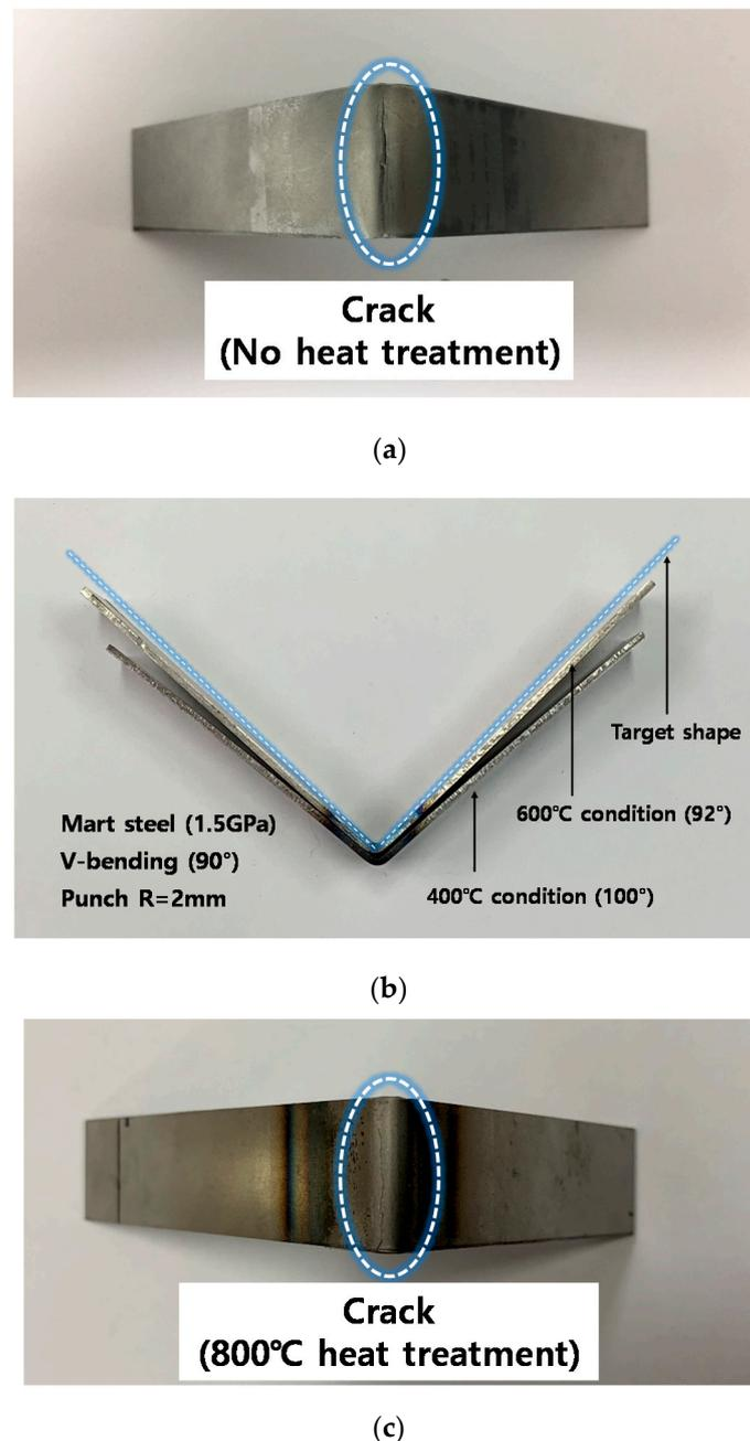
**Figure 5.** V-bending results: (a) Crack on the non-heat-treated specimen; (b) Bent angle; (c) Crack on the 800 °C-treated specimen.
