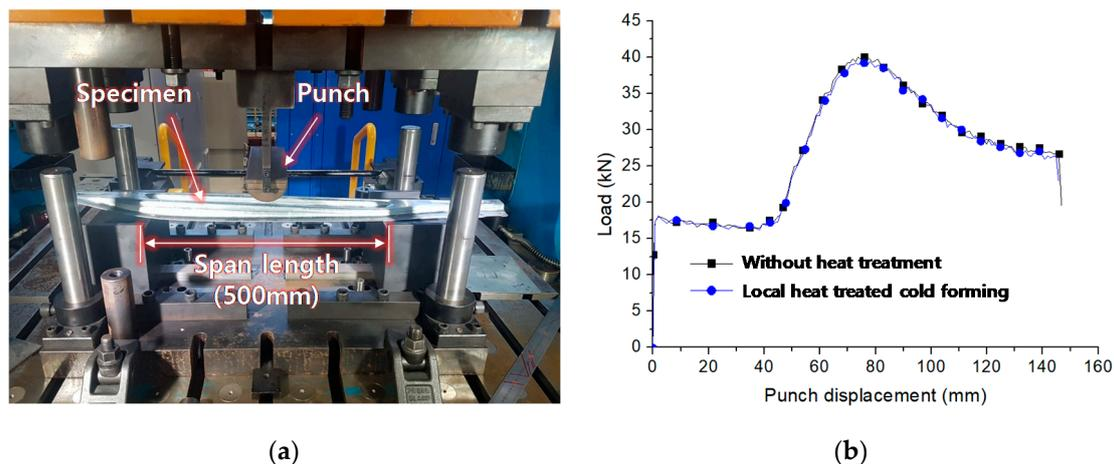
**Figure 14.** Three-point bending test for the door impact beam: (a) Experimental setting; (b) Load–displacement curves.
