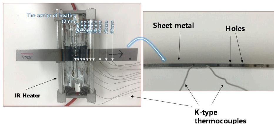
Figure 2. Local heating test.
