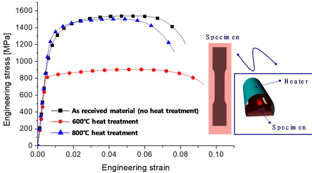
Figure 7. Tensile test after the IR heat treatment.
