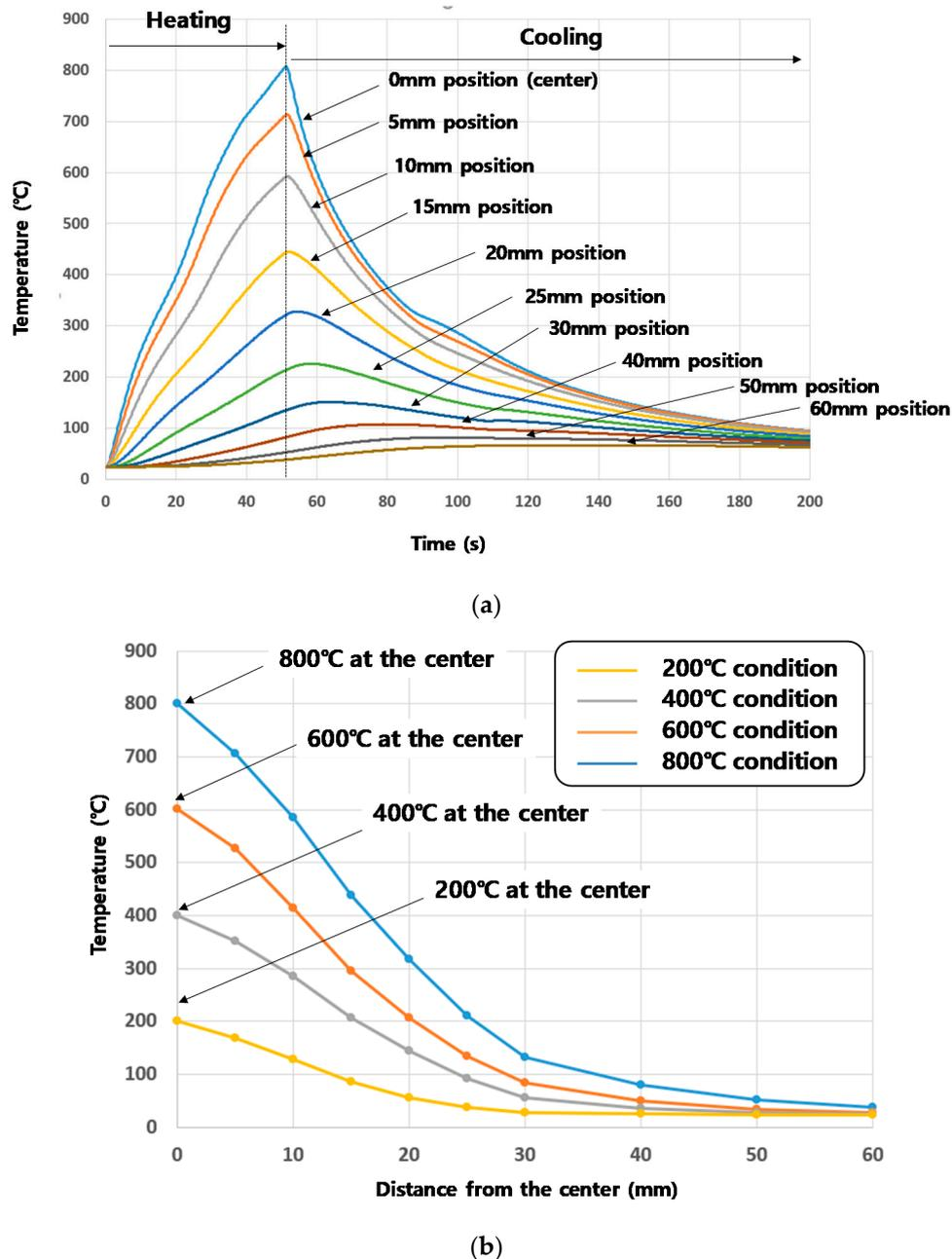
**Figure 3.** Results of the local heating test; (a) Heating and cooling rate at each measurement position; (b) Temperature distributions.
