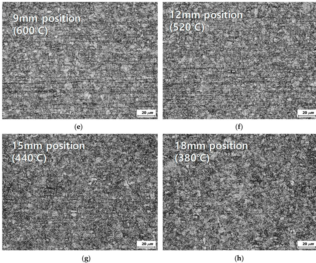
**Figure 9.** Microstructure observation with respect to heated position: (a) As-received material; (b) 0 mm position; (c) 3 mm position; (d) 6 mm position; (e) 9 mm position; (f) 12 mm position; (g) 15 mm position; (h) 18 mm position.
