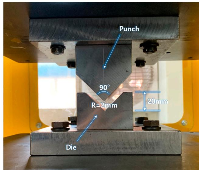
Figure 4. Experimental setting of the V-bending.
