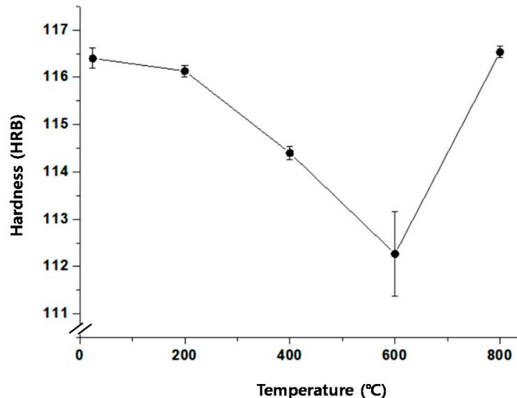
Figure 6. Hardness measurement with respect to the heat-treatment temperature.
