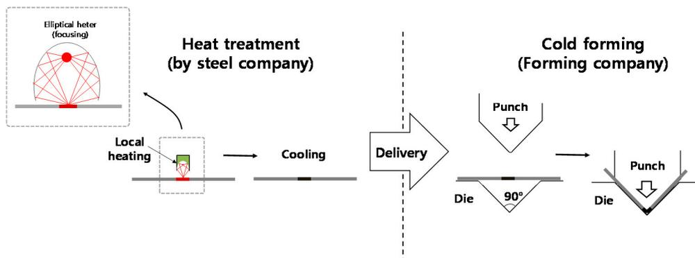
Figure 1. Concept of local heat-assisted cold forming.
