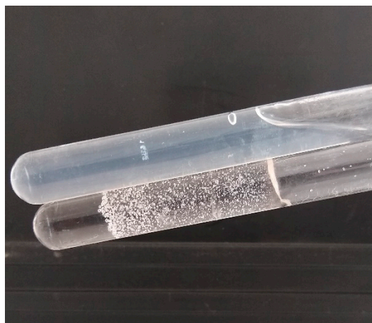
Figure 14. Solution before ( top ) and 30 min after addition of 17.9 M H 2 SO 4 ( bottom ).
