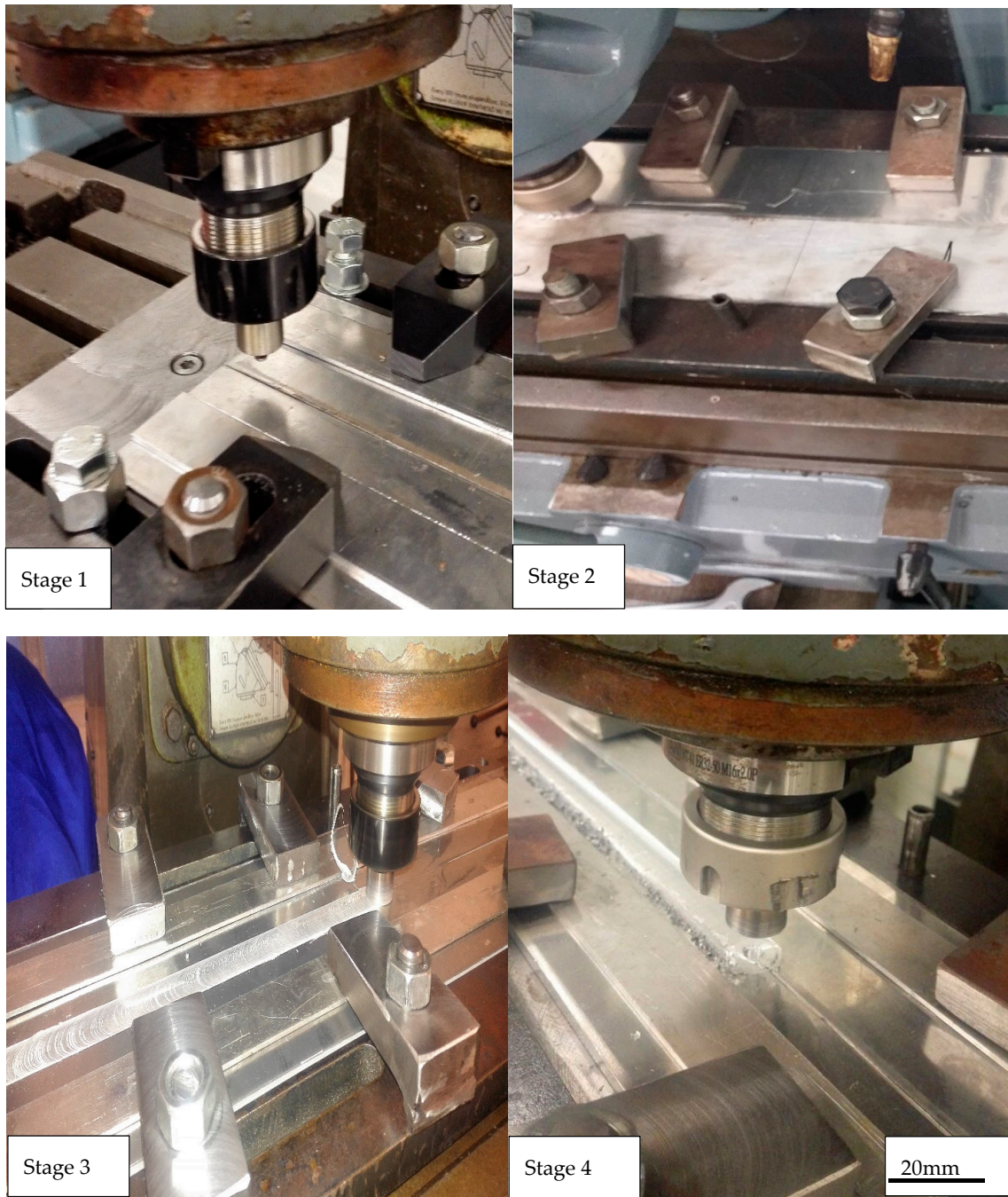
Figure 4. Friction stir welding process.
