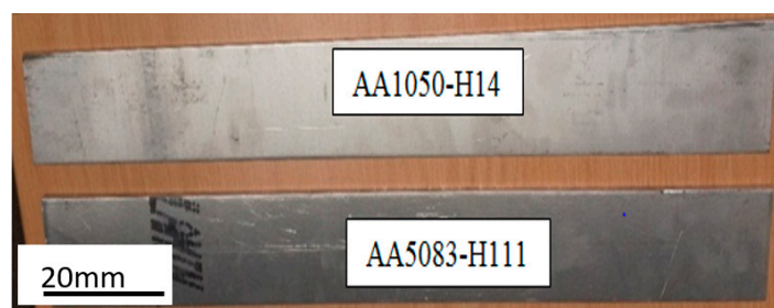
Figure 1. Aluminium alloy plates prepared for welding.
