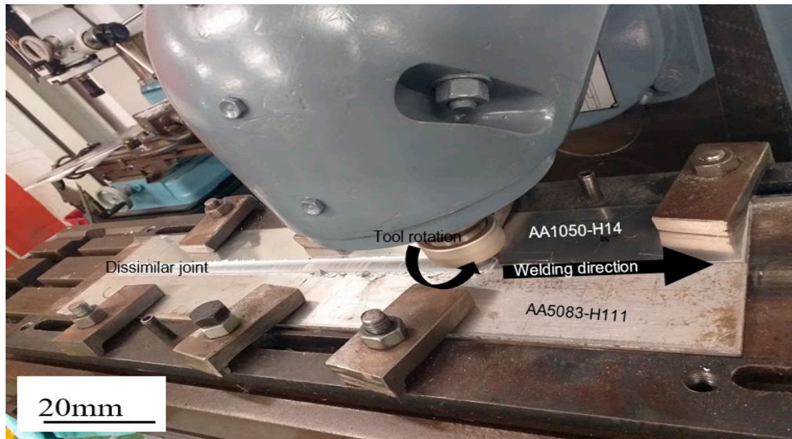
Figure 2. Friction stir welding machine.
