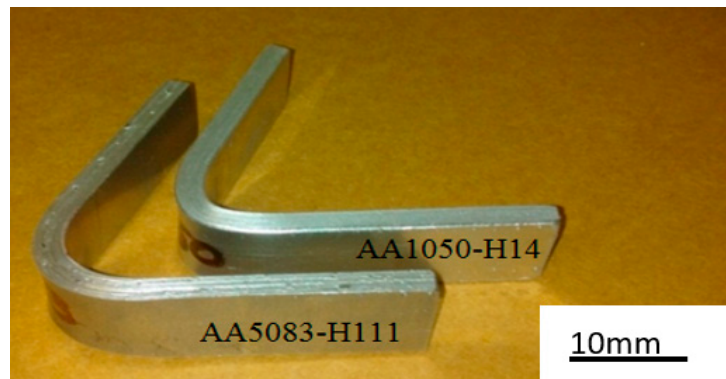
Figure 13. Tested bending specimen (parent materials).
