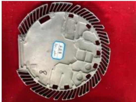
Figure 11. 6063 Al telecom part fabricated by the RheoMetal [130].
