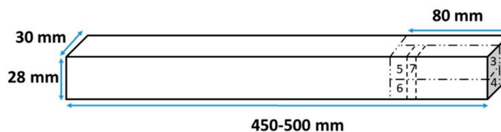
**Figure 1.** Location and orientation of samples in the forged bars. Samples 1 and 2 tensile specimens, 3 and 4 impact specimens, 5 and 6 microstructures, NMI, and HV10 and 7 XRD.
