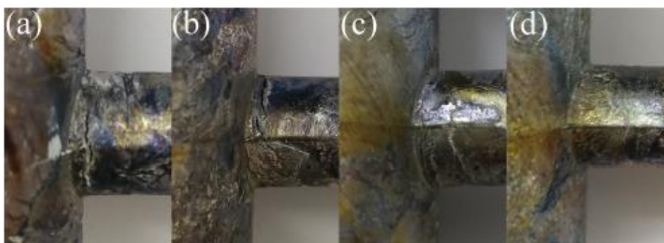
Figure 10. Macroscopic external hot tears of Mg-7Gd-5Y-xZn-0.5Zr alloys: (a) x = 0 wt%; (b) x = 3 wt%; (c) x = 5 wt%; (d) x = 7 wt%.
