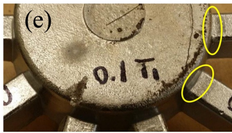
Figure 7. Pictures of representative multi-arm castings with 0.1 wt.% Ti addition: (a) DA1, (b) DA2, (c) DA5, (d) DA6, and (e) DA7.
