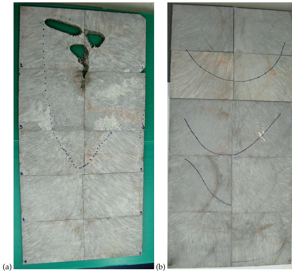
Figure 10. Metallurgical structure revealed on an axial section of the ingot. ((a): top part—(b): bottom part).
