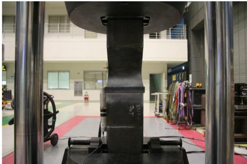
Figure 5. Specimens for direct tensile test at welding joint.
