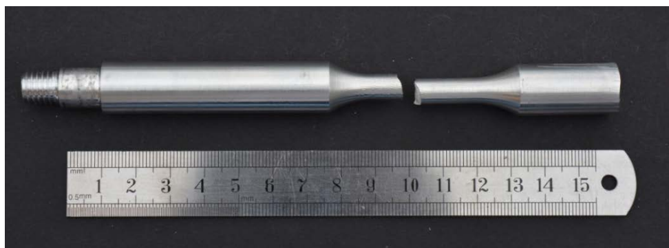
Figure 11. Rotating bar bending test fractured.
