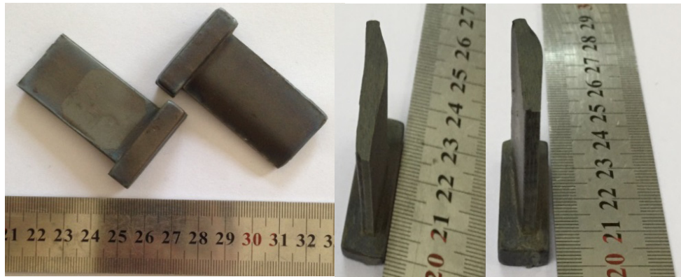
Figure 8. Images of the sandblasted high Nb–TiAl alloy blades.
