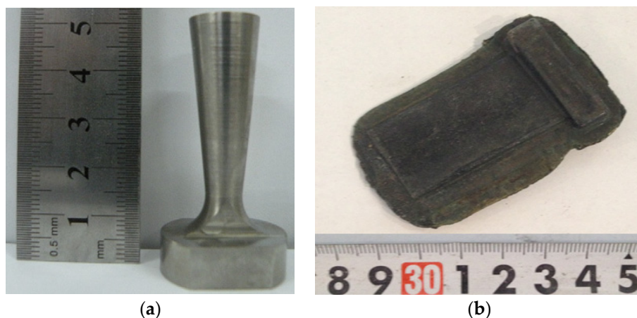
Figure 7. Images of (a) initial billet and (b) high Nb–TiAl blade forged by the isothermal-die.
