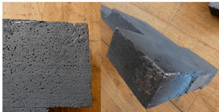
Figure 8. View of the surface where the lustrous carbon defect occurred; Melt 4.
