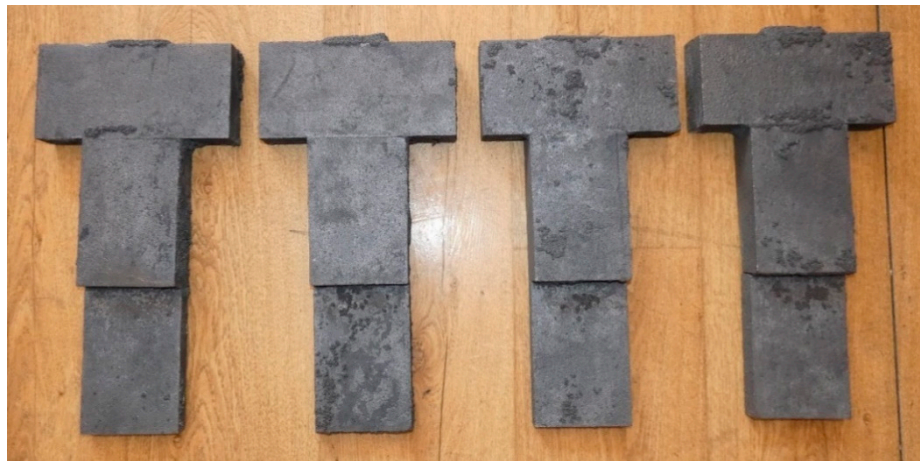
Figure 6. View of castings after removing the inlet system, Melt 3.
