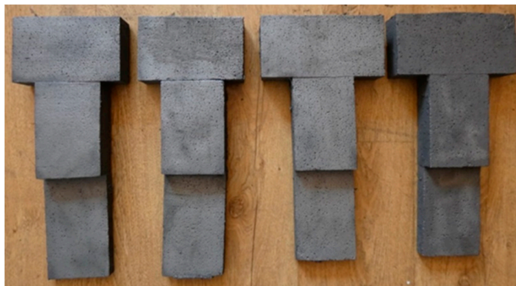
Figure 7. View of castings after removing the inlet system; Melt 4.
