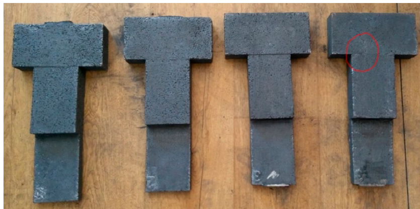
Figure 4. View of castings after removing the inlet system with a marked defect in the form of a lustrous carbon inclusion; Melt 2.
