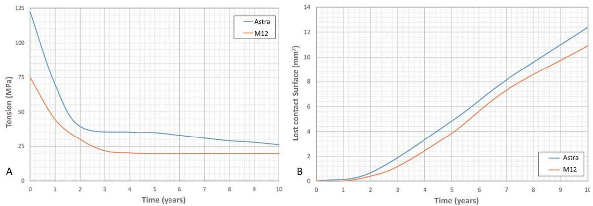
**Figure 3.** Progress of the stress state for the M-12 implant (A). Progress of the stress state for the Astra implant (B). Because of the bone loss, peak stress in the interaction between bone and implant is relaxed. Curves shown in Figure 3 represent the peak stress in the interaction between bone and implant, and it is not related to the same location along the time.
