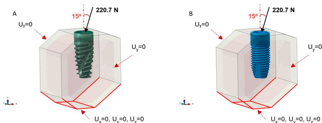
**Figure 1.** Boundary conditions and loading state for the M-12 implant model (A). Boundary conditions and loading state for the Astra implant model (B). The point of application of the load is 5 mm above the implant, affecting the prosthetic abutment, although the implant platform appears directly in the diagram.
