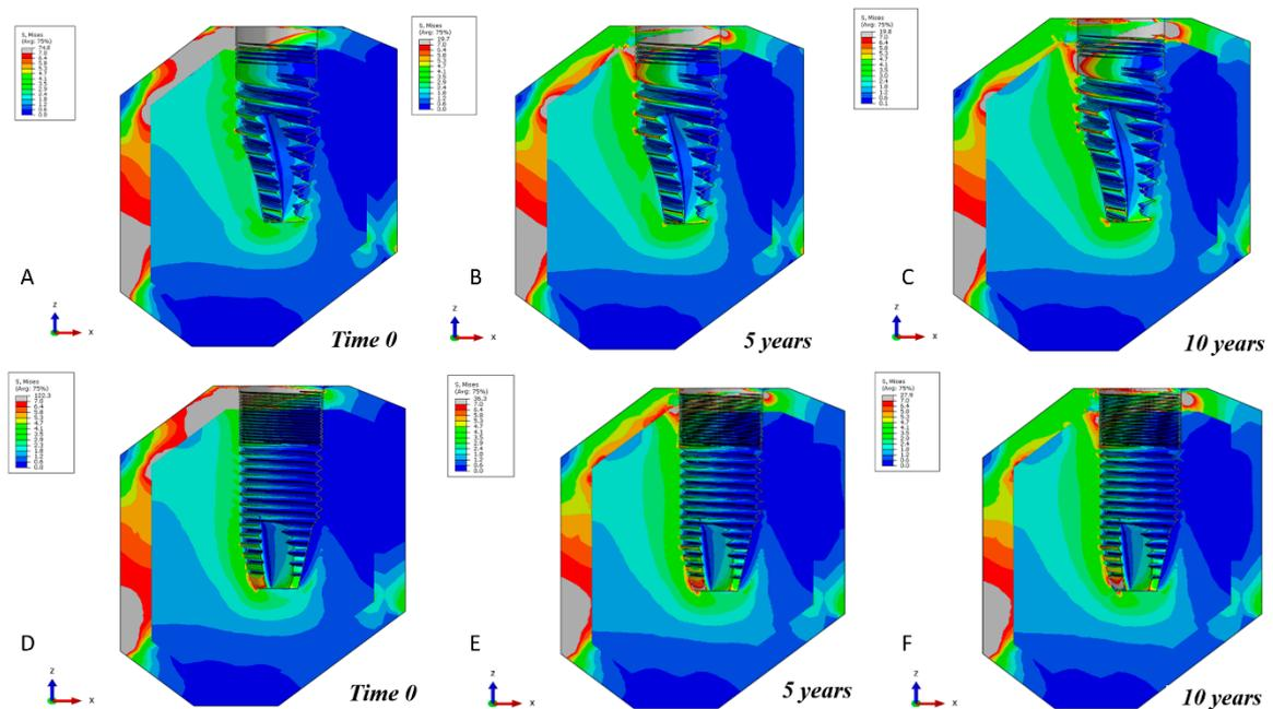
**Figure 4.** Progress of the maximum stress over the 10-year period for the two implants tested in the present study. M-12 implant (A–C). Astra implant (D–F).
