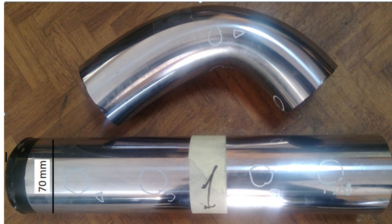
Figure 5. Collected samples from affected and unaffected areas of the rod.
