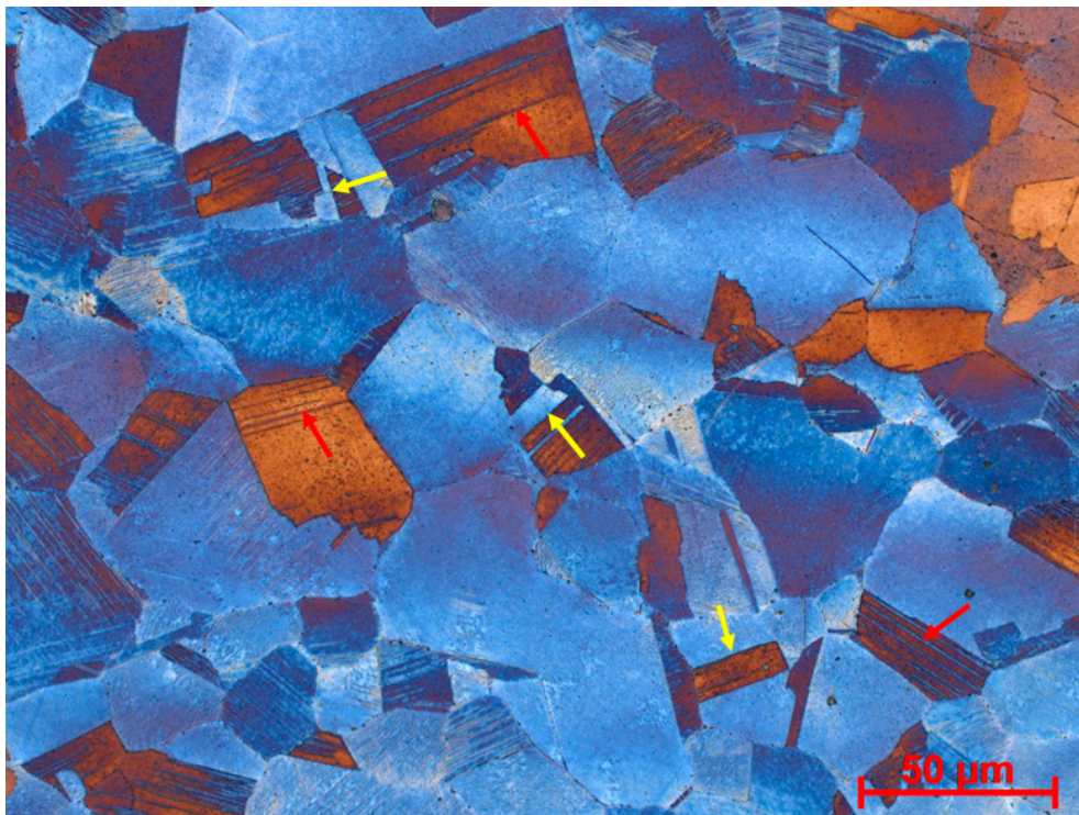
Figure 1. Optical micrograph showing Klemm color etching of the as-quenched Fe-0.9C-17Mn-0.5Si-0.3V-0.019N alloy.
