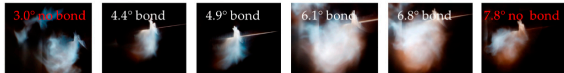
Figure A1. Comparison of the process glare for 1 mm and 1.5 mm flyer thickness at different collision angles, recorded by longtime exposure.
