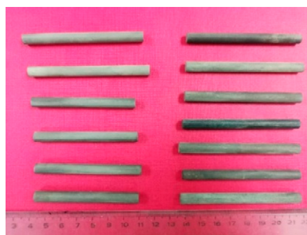
Figure 3. Part of specimens after the uniaxial tensile experiment.
