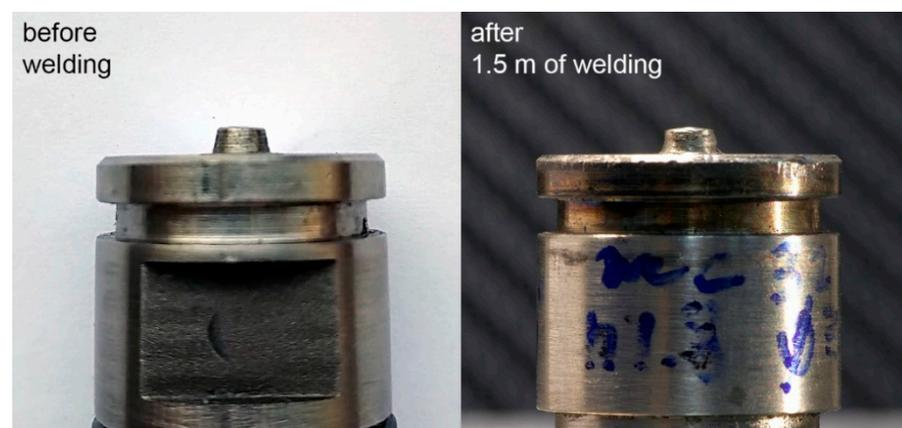
**Figure 14.** Appearance of the tool before and after welding.
