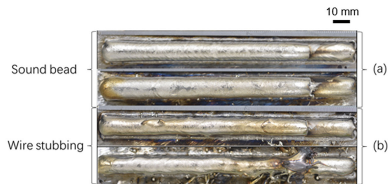
Figure 6. Typical bead appearances. (a) Sound bead and (b) wire stubbing.
