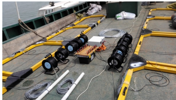
Figure 8. Detection coil and data acquisition equipment.
