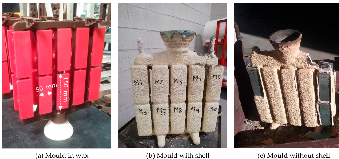
Figure 1. Investment casting moulds in different manufacturing steps.
