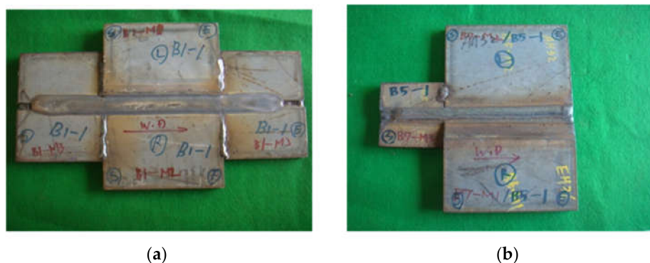
Figure 2. Welding specimens: (a) SAW (B1) and (b) FCAW (B5).
