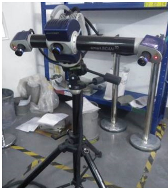
Figure 2. Breuckmann SmartSCAN3D scanner for the warpage measurements.
