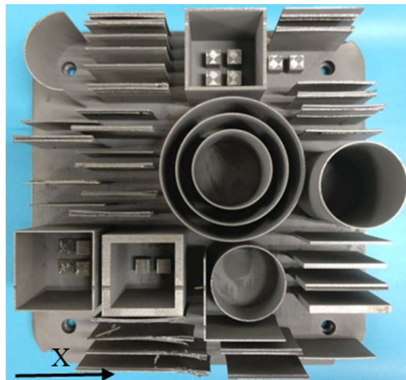
Figure 1. Typical thin-walled structures printed by LPBF.
