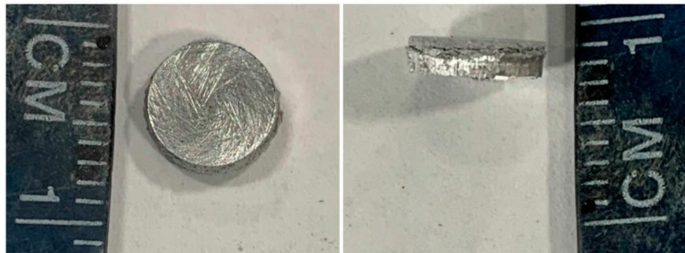
**Figure 12.** Example of aluminum green body formed by compactibility testing.
