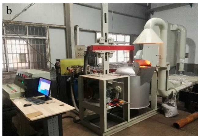
Figure 10. (a) Schematic diagram and (b) image of the electric arc furnace.
