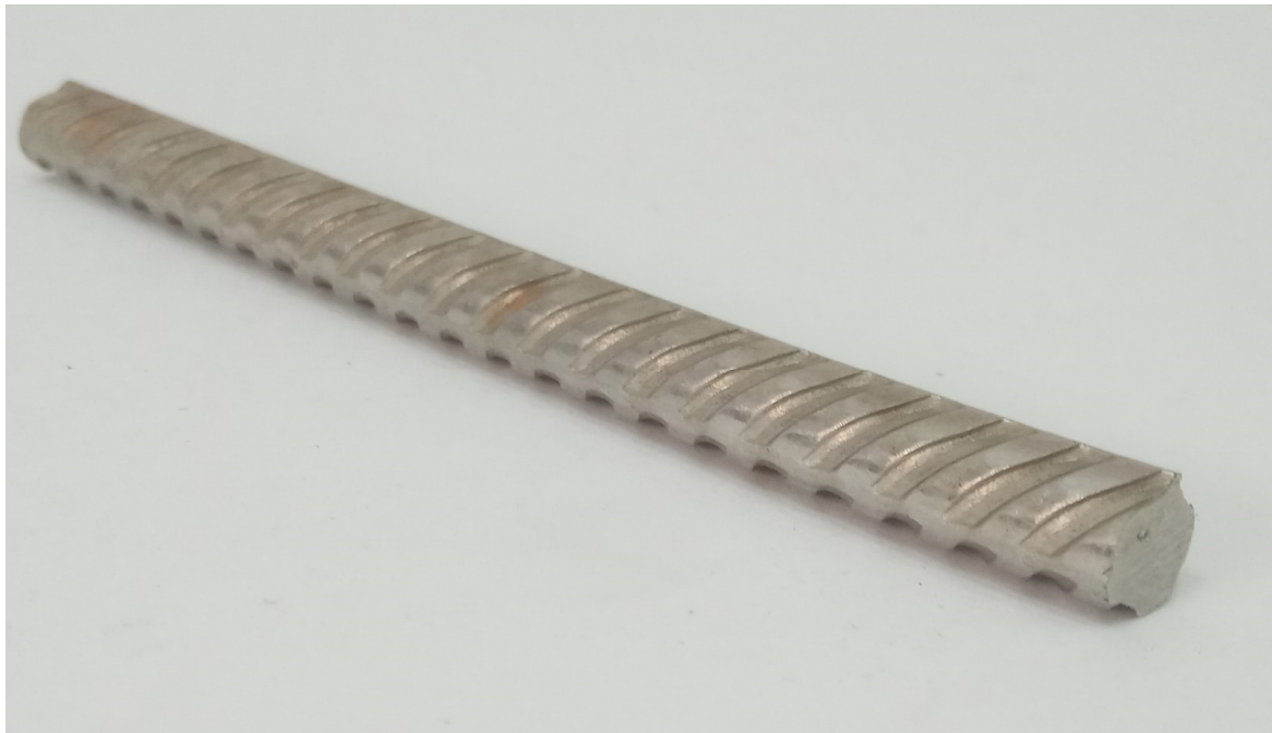
Figure 1. Standard stainless-steel rebar.
