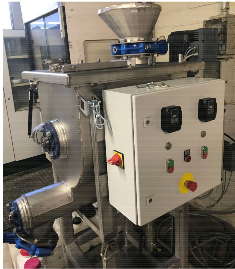
Figure 7. New developed dry digestion reactor (main components: reaction vessel, system with nozzles for injection of water and acid; cover; special mixing system, engine, discharging system, and electronics).
