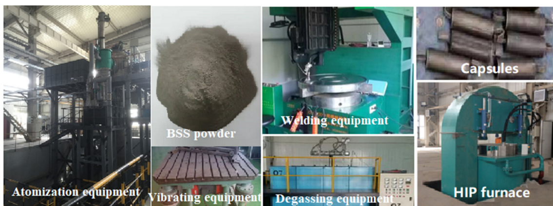
Figure 1. Production equipment, BSS (borated stainless steel) powder, and capsules photographs.
