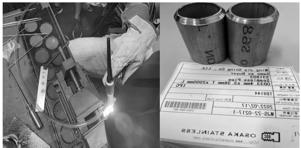
Figure 1. Actual welding diagram of GTAW process for duplex stainless steel pipe.
