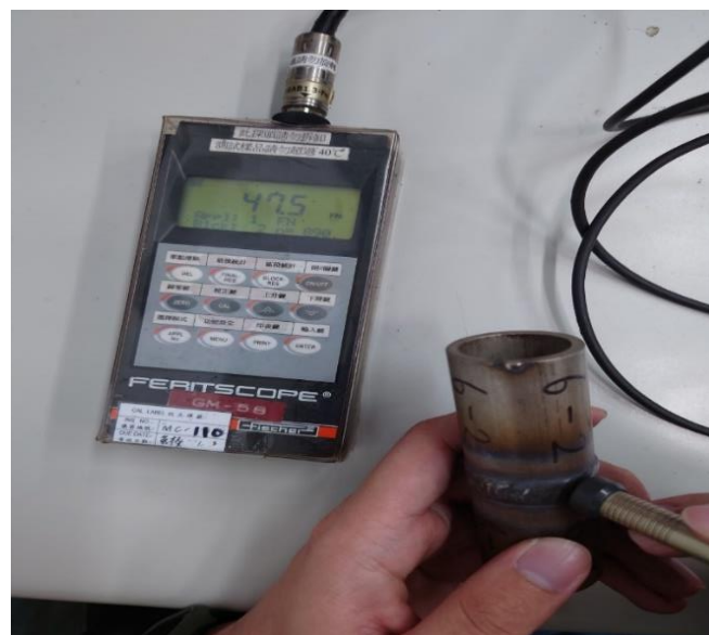
Figure 2. Percentage detection of the test piece with a ferritic rate meter.
