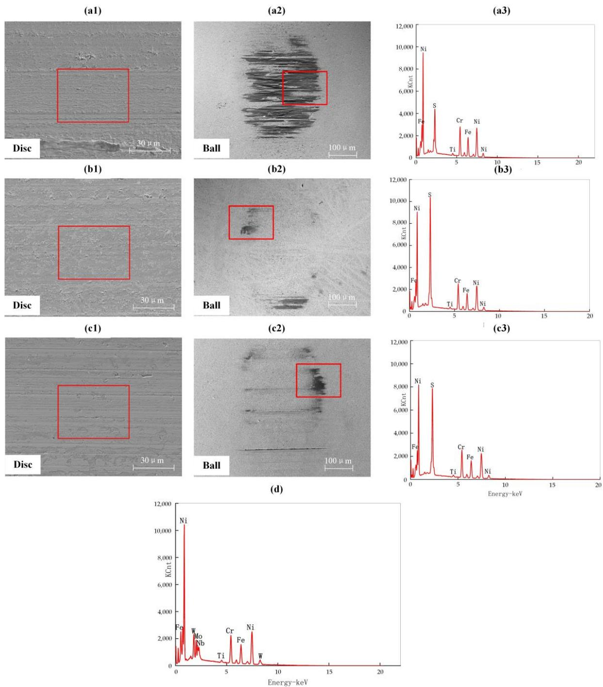
**Figure 5.** SEM morphology of the tracks on Inconel 718 and tungsten carbide ball lubricated under 150 °C lubricated by (a1,a2) sulfurized olefin, (b1,b2) sulfurized fatty acid ester, and (c1,c2) sulfurized lard; (a3,b3,c3) EDS spectrum of the red box in (a1,b1,c1); (d) EDS spectrum of the red box in (a2).
