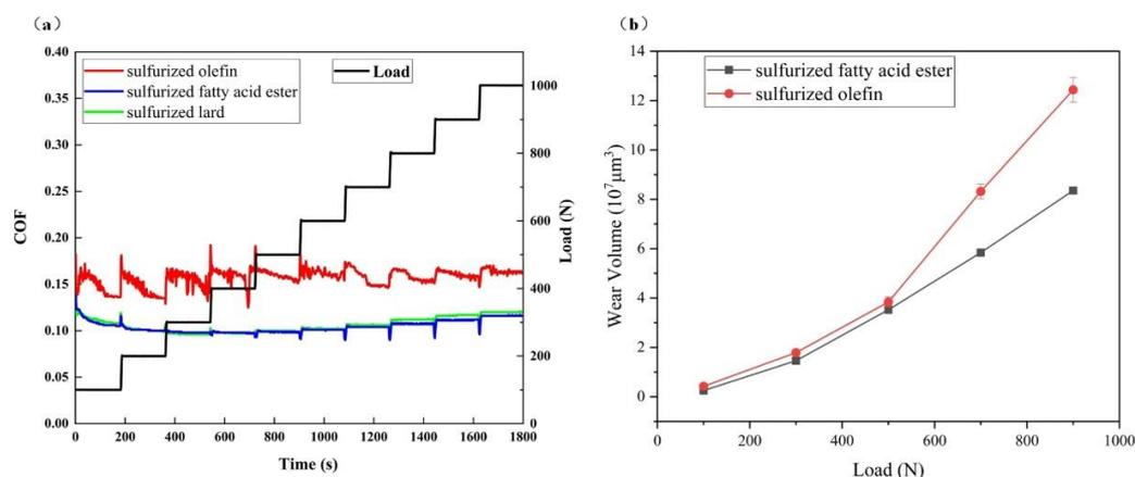
**Figure 6.** (a) Friction coefficient vs. time during a load slope test from 100 N to 1000 N and (b) wear volume under different loads ( $f = 20$  Hz,  $L = 2$  mm,  $t = 25$  °C).
