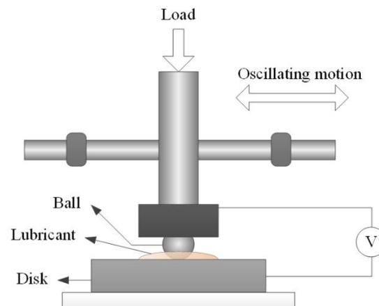
**Figure 1.** The schematic diagram of SRV-IV tribo-tester.
