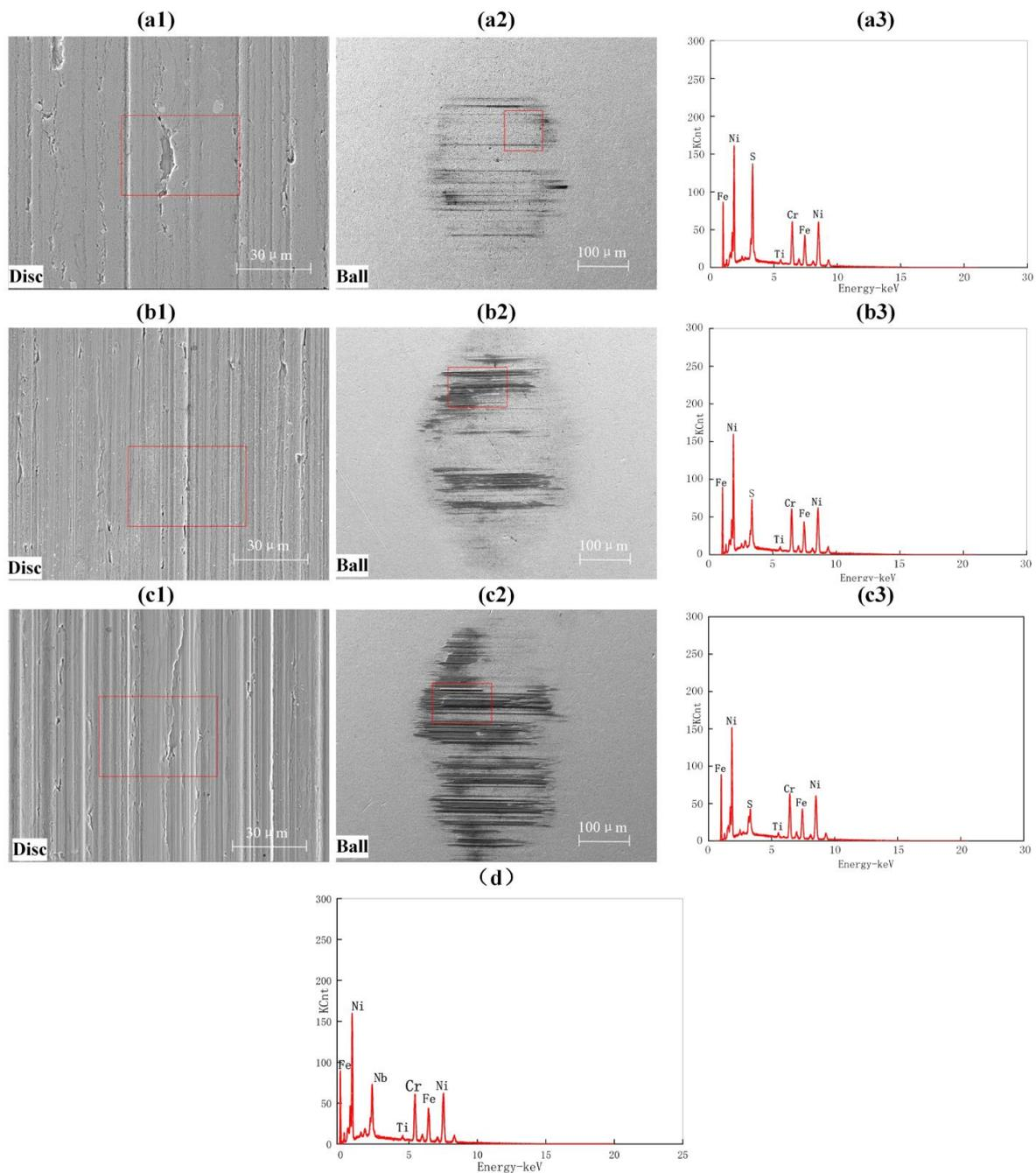
**Figure 3.** SEM morphology of the tracks on Inconel 718 and tungsten carbide ball lubricated by (a1,a2) sulfurized olefin, (b1,b2) sulfurized fatty acid ester, and (c1,c2) sulfurized lard; (a3,b3,c3) EDS spectrum of the red box in (a1,b1,c1); (d) EDS spectrum of the red box in (a2).
