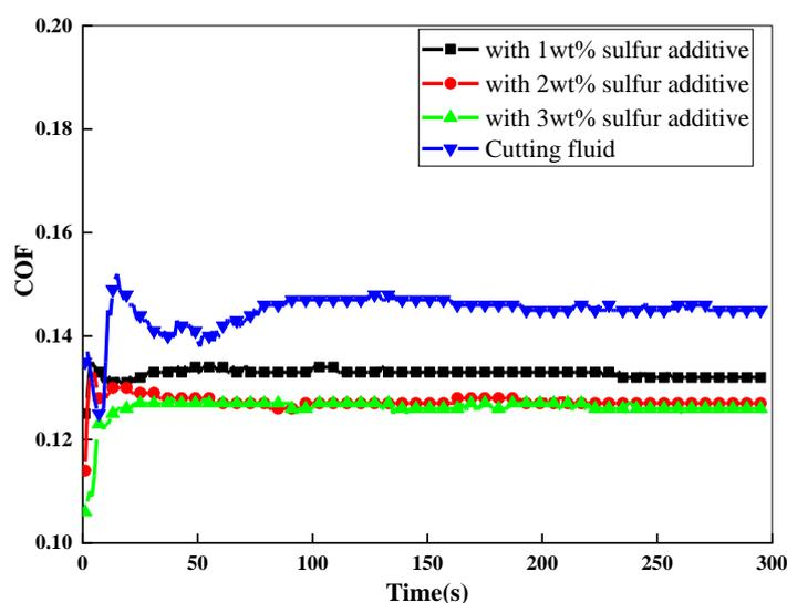
**Figure 9.** The COF of some cutting fluids with different contents of sulfurized fatty acid ester ( $F = 100$  N,  $f = 20$  Hz,  $L = 2$  mm,  $t = 25$  °C).
