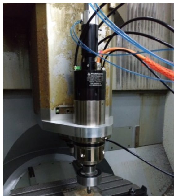
Figure 3. Coaxial laser-assisted spindle of the CNC milling machine.
