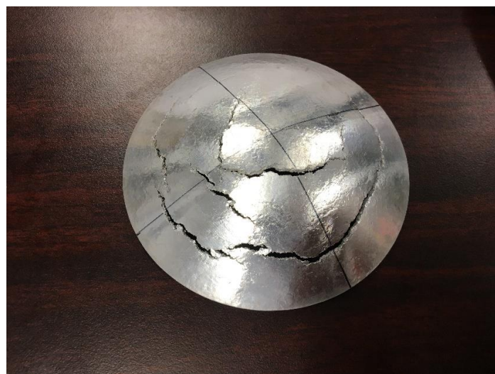
Figure 19. Cracked AZ91 plate obtained when using a hyperbolic pressure vessel with a charging voltage of 2000 V and sandwiched between auxiliary plates.
