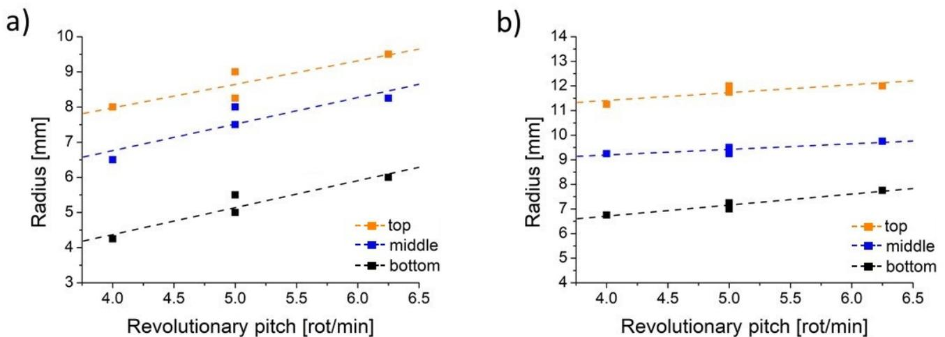
**Figure 8.** Radius of the nugget zone as a function of revolutionary pitch—relationship for the friction stir welds produced with the tilt angle 0° (a) and 2° (b).
