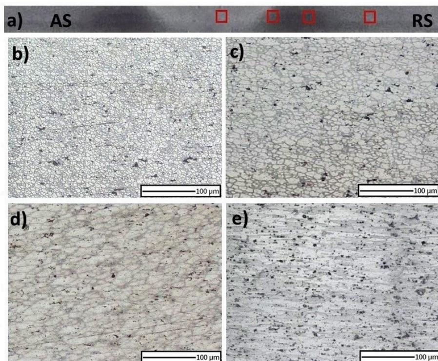
**Figure 4.** Macrostructure of FSW7 sample with the locations of microscopic observations (a) and its microstructures observed in the nugget zone (b), thermo-mechanically affected zone (c), heat-affected zone (d), and the microstructure of the base metal (e).
