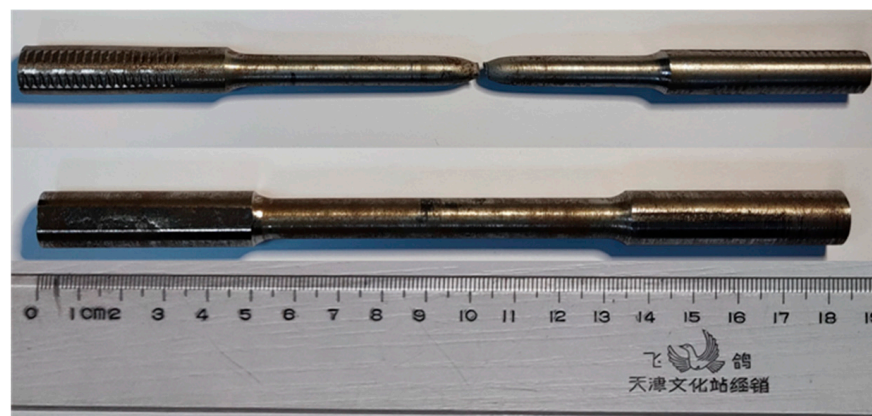
Figure 3. Specimen with a circular section before and after the material test.
