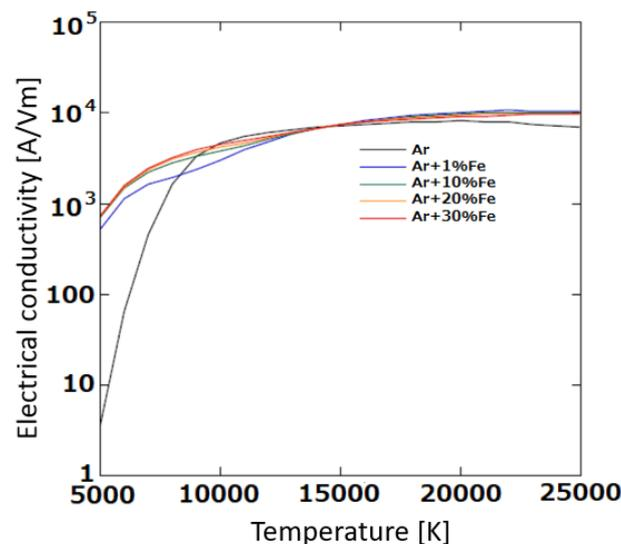
Figure 7. Dependence of electrical conductivity on temperature and metal vapor concentration.
