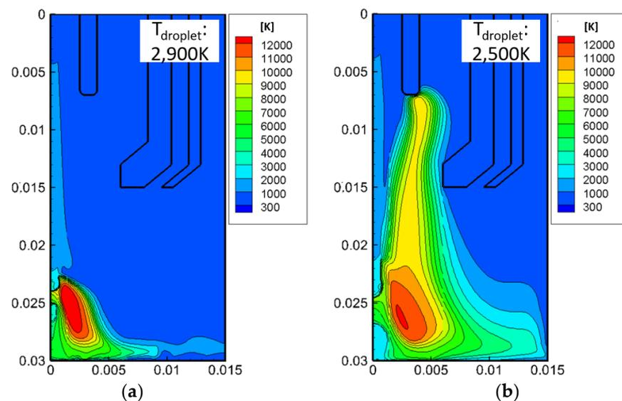
Figure 3. Temperature distributions in (a) conventional MIG welding and (b) plasma–MIG welding.
