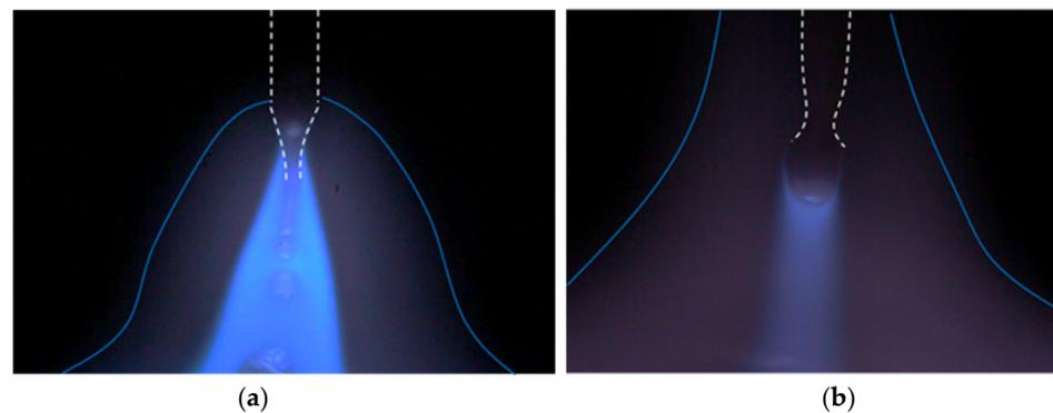
**Figure 1.** Arc and plasma appearance in (a) conventional MIG welding and (b) plasma-MIG welding.
