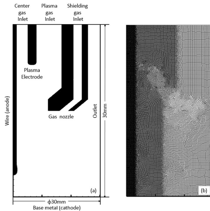
Figure 2. (a) simulation region and (b) mesh.
