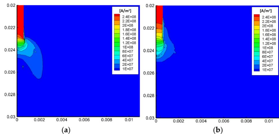
**Figure 6.** Current density distributions in (a) conventional MIG welding and (b) plasma-MIG welding.
