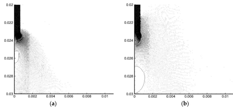
**Figure 5.** Current density vectors in (a) conventional MIG welding and (b) plasma-MIG welding.
