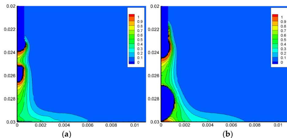
Figure 4. Metal vapor mole fraction distributions in (a) conventional MIG welding and (b) plasma–MIG welding.
