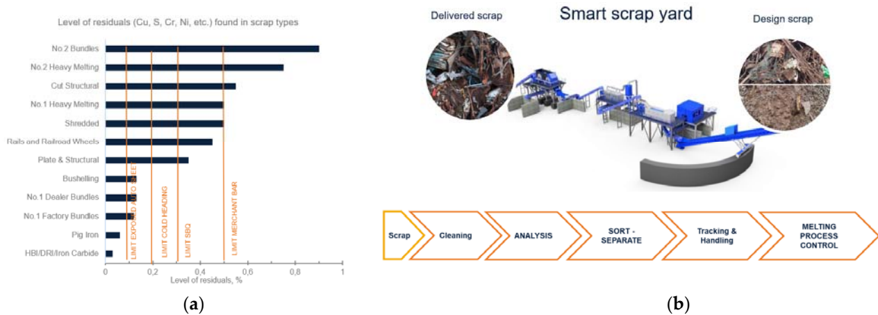
Figure 3. (a) Residual element level for different scrap types and limits for steel groups (b) Overview scrap processing plant and different process steps.
