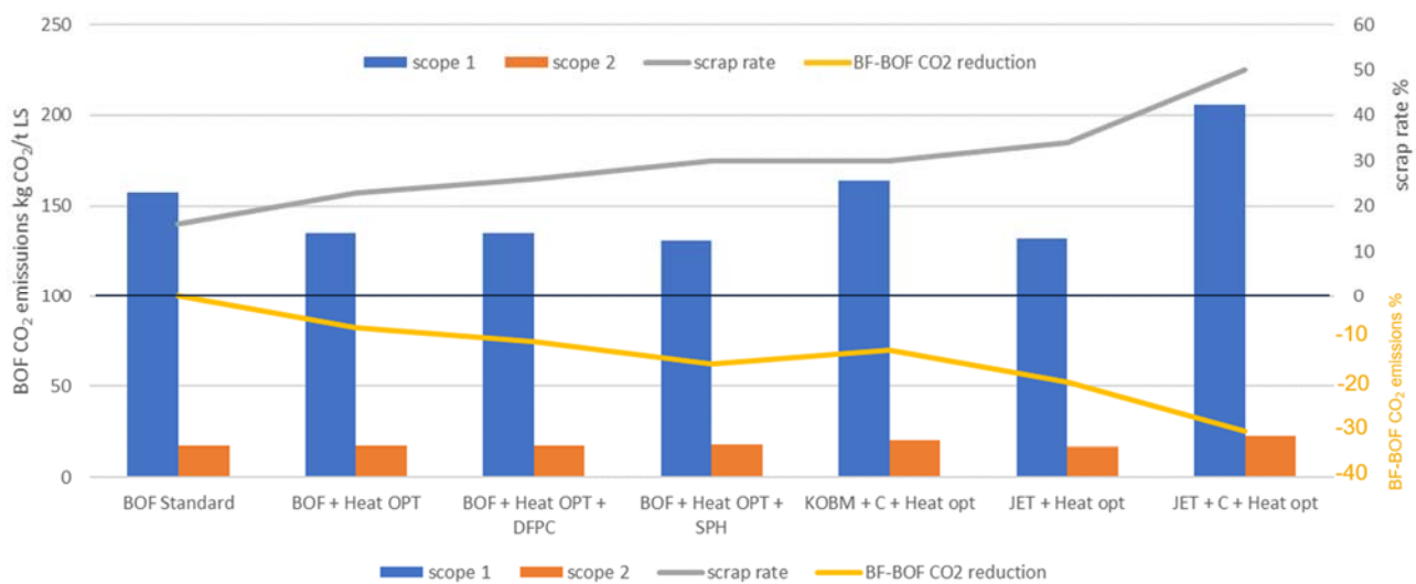
Figure 14. Specific CO 2 emissions (scope 1 and scope 2) per ton of liquid steel (LS) for different BOF solutions, including possible scrap rate and potential for reduction in total BF–BOF CO 2 emissions. Variation depending on operation conditions possible.
