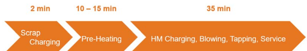
Figure 8. Typical processing time for BOF with scrap preheating.
