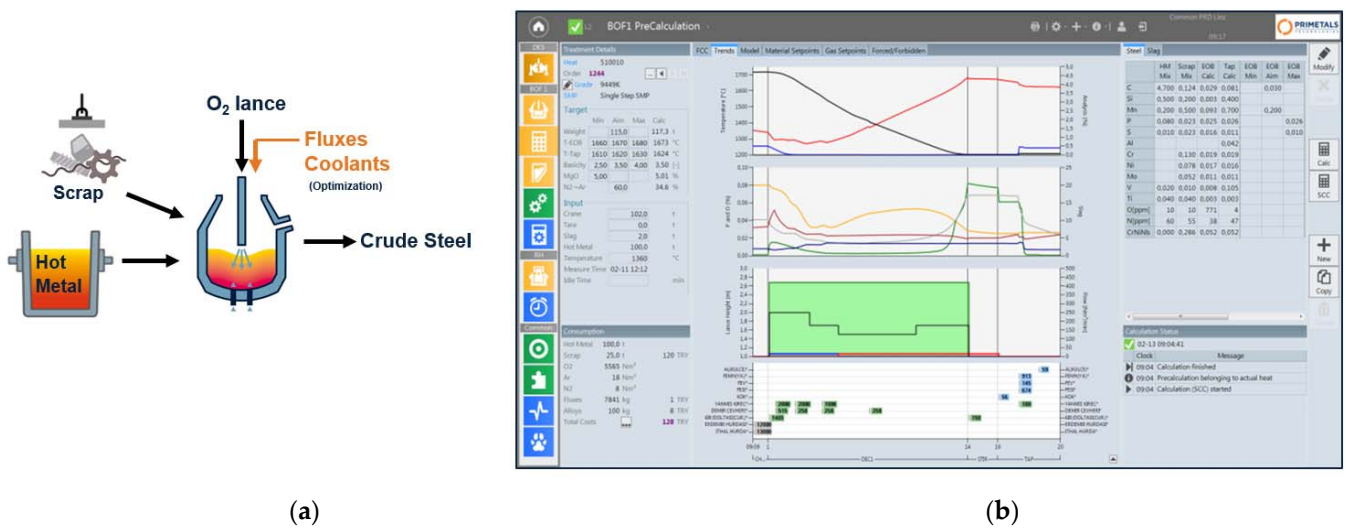
Figure 6. (a) Heat optimization through replacement of cooling additions with scrap. (b) Interface of Level 2 process model for process simulation and control. The calculated temperature (red), carbon (black), and silicon content (red) are shown in the middle-upper diagram. Slag composition, blowing pattern, and material addition schema are illustrated in the lower diagrams.
