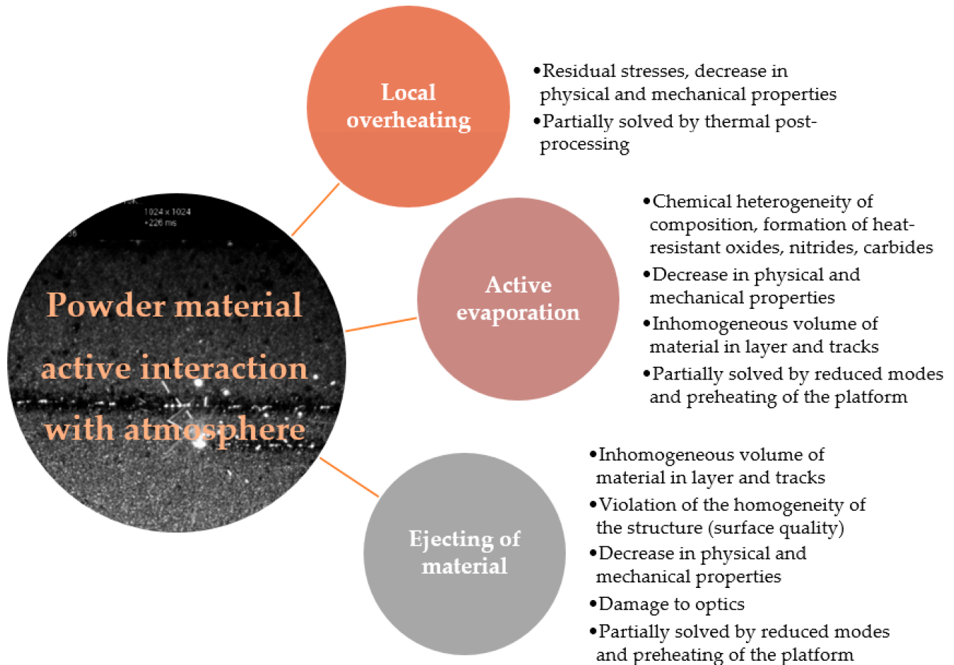
Figure 1. The main consequences of the active interaction of powder material with atmosphere and the existing ways of solving them.
