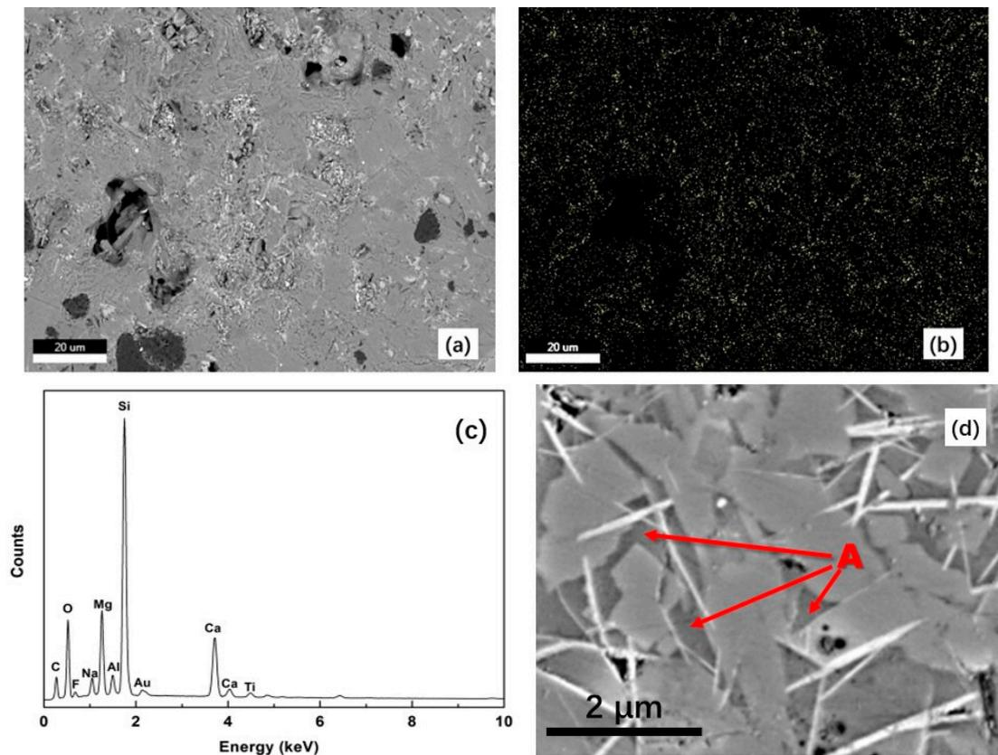
Figure 5. Typical backscattered electron image of final slag (a), distribution of Ti-bearing phase (b), and EDS analyses of the Ti-bearing phase (c). Ti-bearing phase (A) is in an amorphous state that is dispersed in solidified slags (d). Sample obtained in slag with basicity index of 1.4.
