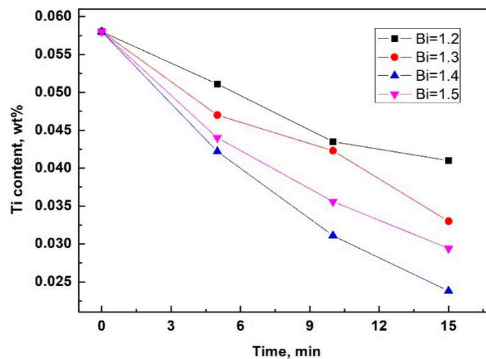
**Figure 1.** Ti contents of metallurgical-grade silicon during refining (using slags with different basicity indices).
