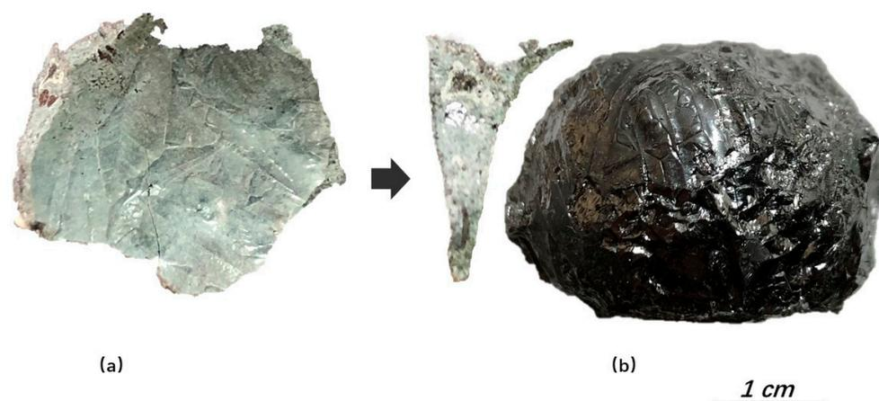
**Figure 3.** Solidified surface of slag that contacted with silicon (a) and cross-section of solidified slag and the contacted silicon lump (b).
