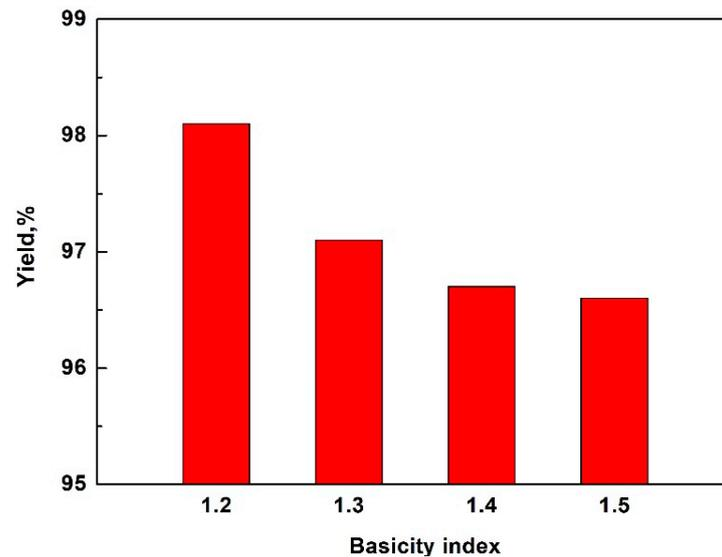
Figure 4. Effect of basicity index of slags on the yield of silicon after 15 min of refining.
