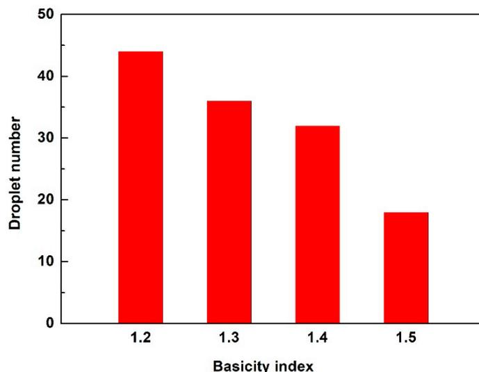
**Figure 2.** Effect of slag basicity index on the overall number of silicon droplets at the silicon–slag interface (inspection area: 1 mm × 1 mm).
