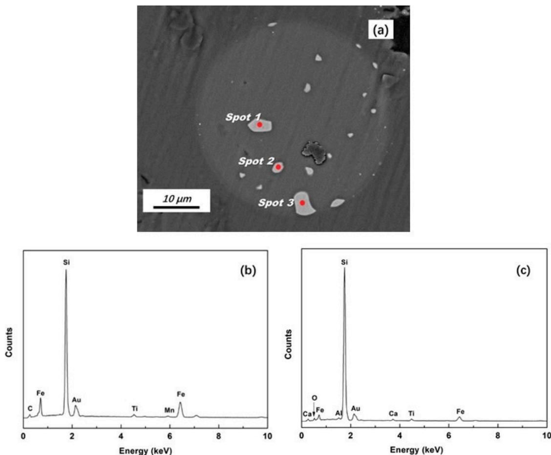
**Figure 6.** A typical backscattered electron image of silicon droplet in slag (BI = 1.4) near silicon–slag interface (a); EDS analyses at spot 1 (b) and spot 3 (c).
