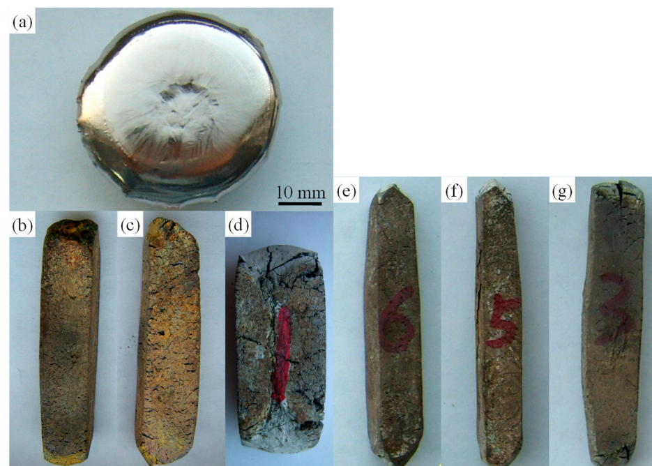
Figure 1. The morphologies of the 60 g ingot (a) and open-forged specimens (b–g). (a) 60 g ingot; (b) 2Zr-4O alloy; (c) 2Zr-6O alloy; (d) 2Zr-10O alloy; (e) 0Zr-4O alloy; (f) 0Zr-6O alloy; (g) 0Zr-10O alloy.
