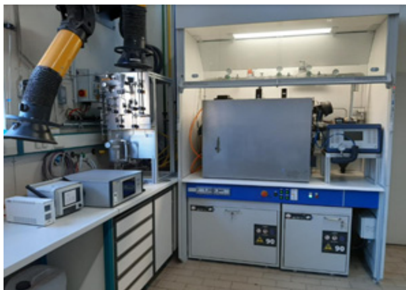
Figure 5. Online conditioning and analysis system of ALFE_CH3OH_PLP.
