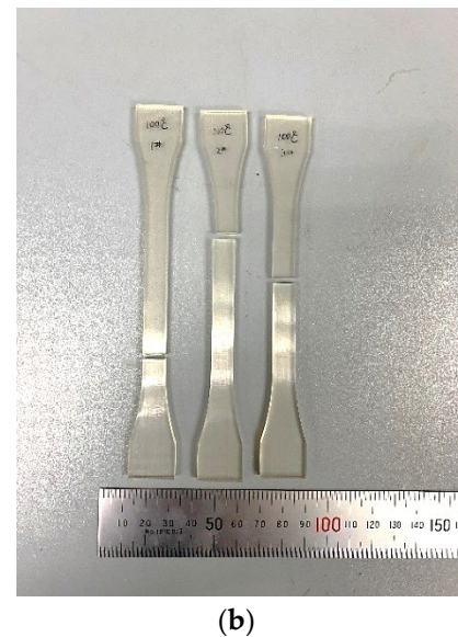
Figure 5. The uniaxial tensile test results of the metallized acrylic containing 5 wt % \text{Gd}(\text{MAA})_3 and 30 wt % \text{Pb}(\text{MAA})_2 at 100 °C. (a) The true stress–strain curves under different strain rates. (b) The fractured metallized acrylic specimens after tensile test at 100 °C.
