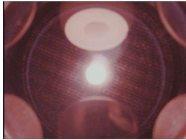
**Figure 1.** A positively charged sample levitating among 3 pairs of electrodes in the ISS-ELF.
